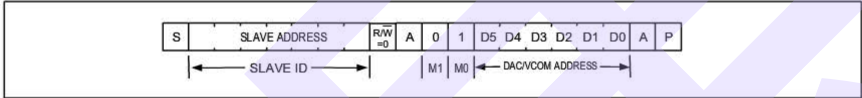
Figure 13. Single Acquire Command to Update One Output with MTP
