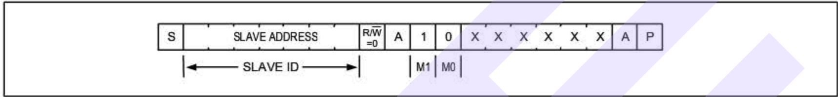
Figure 12. General Acquire Command to Update All Outputs with EEPROM
