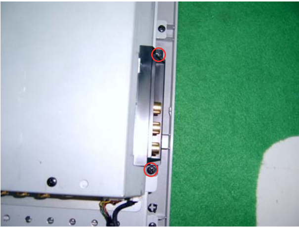
4. Remove 2 screws from the side connector. Lift up the shield-cover.
