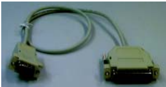
Fig. 1 => ISP CABLE : 12nc is "3138 106 10148".
