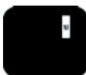
Three adjacent lit subpixels (one white pixel)
