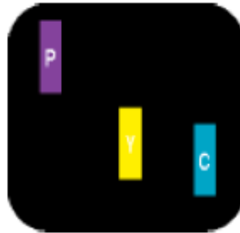
Two adjacent lit sub pixels: - Red + Blue = Purple - Red + Green = Yellow - Green + Blue = Cyan (Light Blue)
