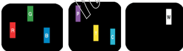
Two adjacent lit sub pixels: - Red + Blue = Purple - Red + Green = Yellow - Green + Blue = Cyan (Light Blue)
