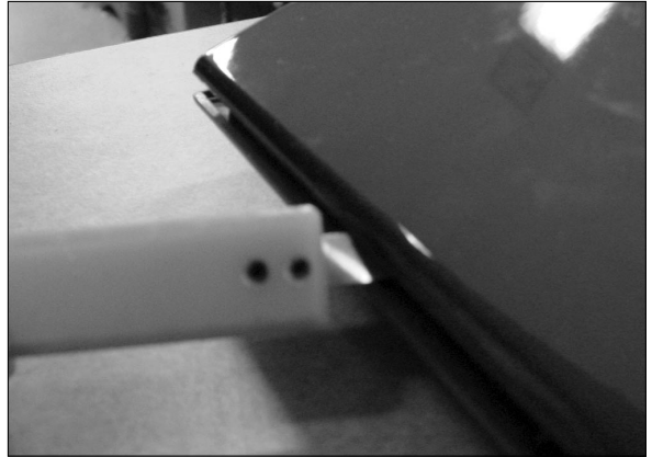
Open the Backcover's latch with Jig.
