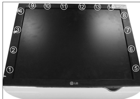
Unlock Latch between C/A and B/C as 1~14 sequence.
