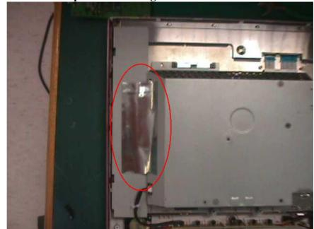
Q. Paste aluminum tape on the backlight wire hole
