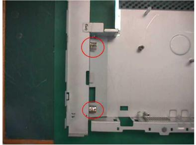
B. Screws on the interface & power board
