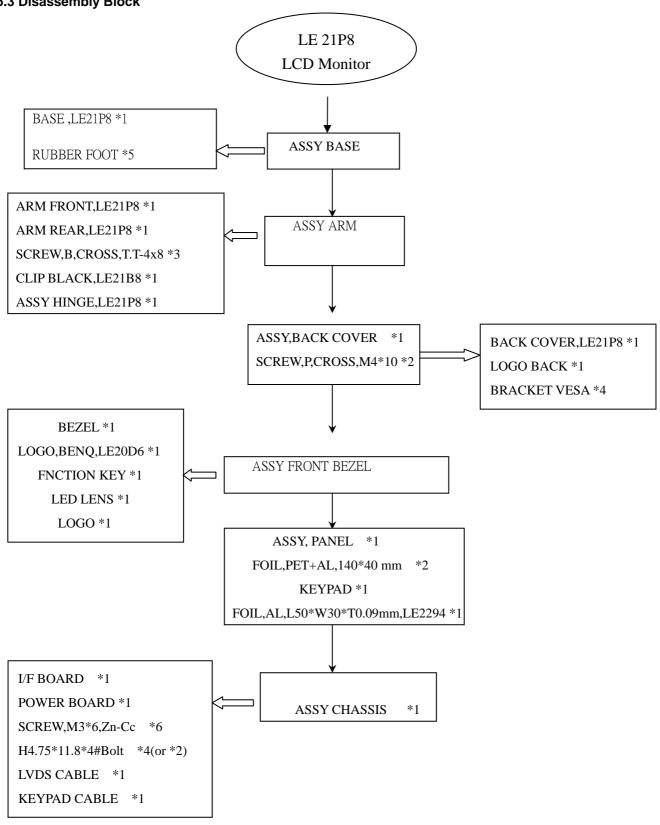
Note: The disassembly direction please following direction of arrowhead
